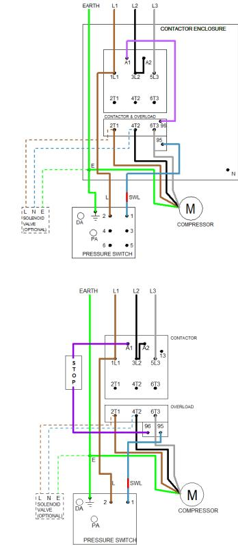
Notes: Solenoid unloader valve is optional (standard with low pressure switches) Wiring colours may be different from those stated for older models Based on Danfoss CS-type pressure switch (your switch may be different)
