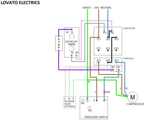
Notes: Solenoid unloader valve is optional (standard with low pressure switches) Wiring colours may be different from those stated for older models Based on Danfoss CS-type pressure switch (your switch may be different)
