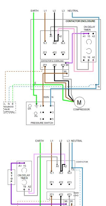
Notes: Solenoid unloader valve is optional (standard with low pressure switches) Wiring colours may be different from those stated for older models Based on Danfoss CS-type pressure switch (your switch may be different)
