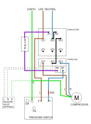
Notes: Solenoid unloader valve is optional (standard with low pressure switches) Wiring colours may be different from those stated for older models Based on Danfoss CS-type pressure switch (your switch may be different)
