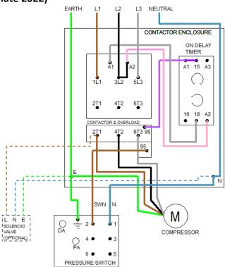
**Notes**: Solenoid unloader valve is optional (standard with low pressure switches) Wiring colours may be different from those stated for older models Based on Danfoss CS-type pressure switch (your switch may be different)
