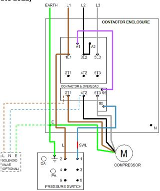
**Notes**: Solenoid unloader valve is optional (standard with low pressure switches)
