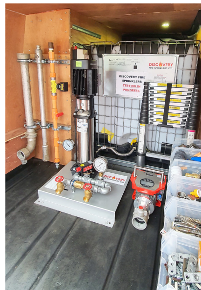
Dry Riser Test Pumps installed in customers' vans
