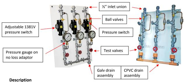
This compact, lightweight modular pump test assembly is designed to meet the requirements of LPC and BS5306. 'Single' switch models only for Wet Riser (or some older sprinkler systems).
